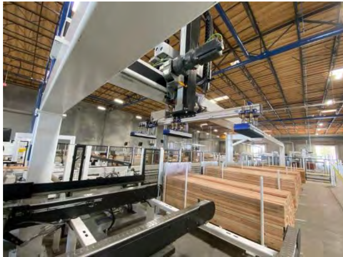
Photo 17- Entekra LLC fully automated off-site construction
