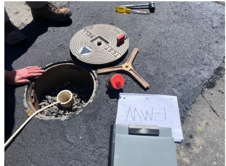
Measuring Static Water Level at MW-1S
