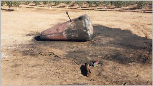
"Damaged tank from explosion: Tank ends are bowed outward. No emergency venting evident. Small grinder with wire brush wheel nearby."—Hank Moore, Merced County Fire Marshal
