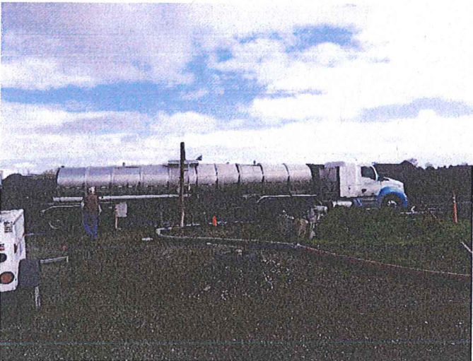
Figure 17 A tanker truck being filled for off-hauling of leachate from the West Pond to the East Bay Municipal Utility District.
