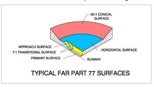
ends of runways having a precision instrument approach. The FAA conducts an aeronautical study of proposed construction and determines whether the use would be a hazard to air navigation. The evaluation considers only the height of the proposed structure(s). The FAA may recommend removal, marking, or lighting the obstruction(s). The Airspace Plan consists of Sheets 3 and 4.
