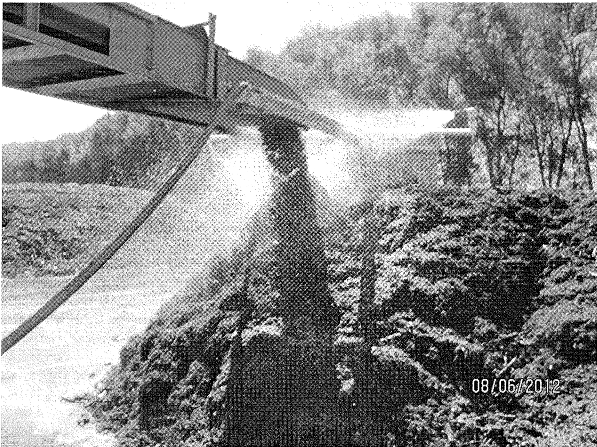
Photo 3: Water sprayer system wetting composting feedstock as they are discharged from the potato piler.
