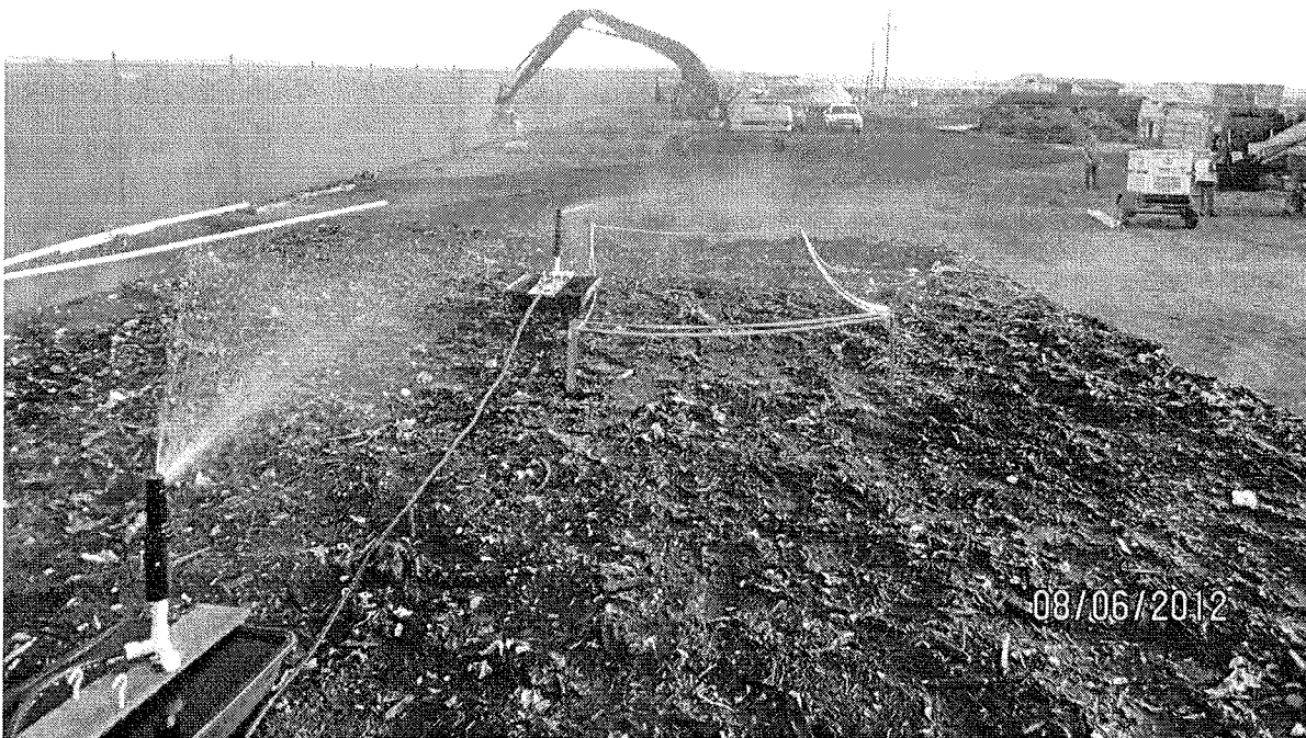
Photo 4: Irrigation sleds wetting top of prototype eASP. Note- test areas cordoned off for air emissions sampling.
