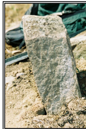
Witness corner located in Section 30, T.7S., R.7E
