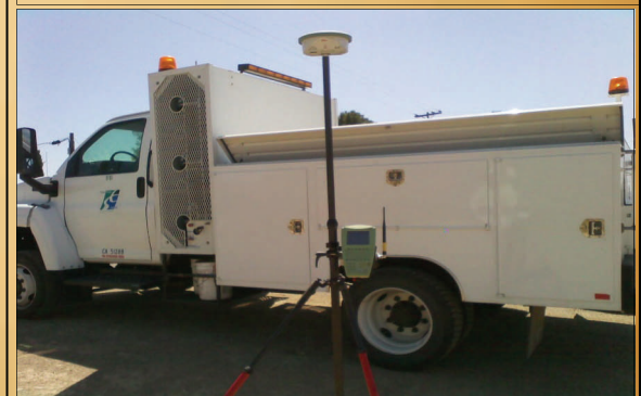
Leica GPS Rover Unit (Model 1200 Series) in front of County Survey Truck #1111, circa 2012
