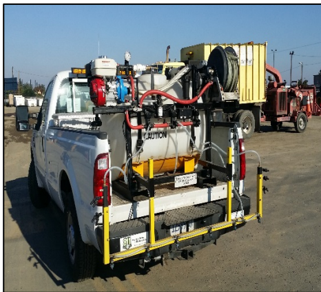
Chemical Spray Skid
