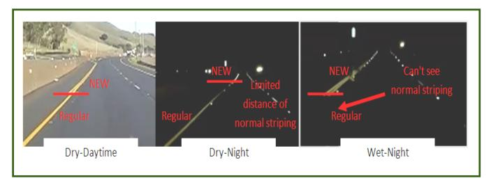
High performance striping material versus regular striping material
